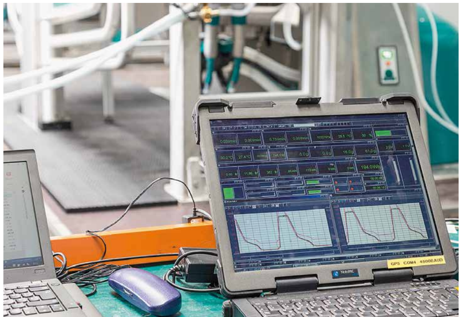
By replicating various milk flow rates, the DLG measures electricity consumption relative to the milking performance of the cows. The difference between one- and two-box electricity use is surprising.
