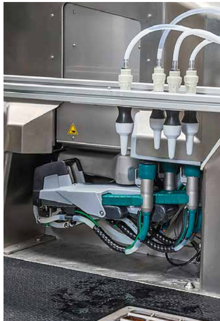
Teat cleaning and dipping operations take place inside the teat cups on the GEA DairyRobot.
